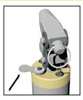
**6.** Prime the pump and advance the wedge forward.
