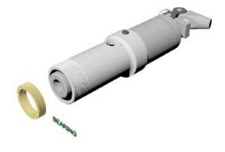
**4.** Remove the piston rod, seal and spring.
