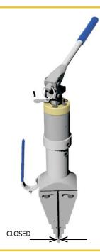
**14.** Close the release lever and prime the wedge open.
