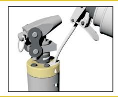
**5.** Close the release lever in a clockwise direction.
