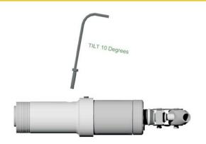
Screw the socket cap screw at this angle through the spring until it will screw no further.
