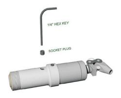
**2.** Using an M5 hex key unscrew and remove the socket cap screw.
