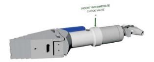
Place a 5mm flat punch in top of the check valve and hold firmly with one hand. Ensure that the punch is held vertically and, using a hammer, apply one firm blow to the punch.
