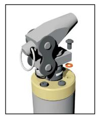
**3.** Use an oil can which has been cleaned and filled with hydraulic oil (Grade 32 centi).
