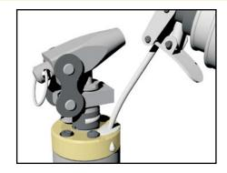
**9.** Open the release lever slowly allowing the wedge to retract. As the wedge retracts hydraulic oil and air bubbles will over-flow out of the filler hole.
