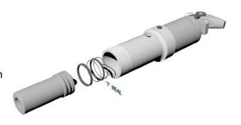
**6.** Ensure that the spring is inserted at 90 degrees to the socket cap screw as it is placed into the pump.
