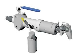
**7.** The pump should be held in a vice and the body can then be unscrewed using a monkey wrench or stillson.
