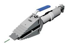
**4.** Remove the M6 x 12 mm grub screw from the wedge.
