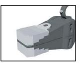
**1.** Attach the stepped block to the tool using the M6 countersunk screw
