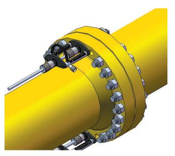
**19.** The FC10TE can now be removed by gripping and pulling on the pull sleeve section of the primary nut.
