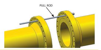
**2.** The FC10TE Tool is slid over the pull rod untill the face of the tool comes into contact with the flange.
