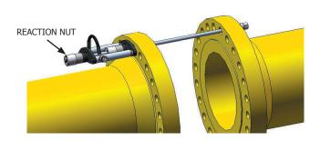
**4.** The hydraulic hand pump and Hoses are connected
