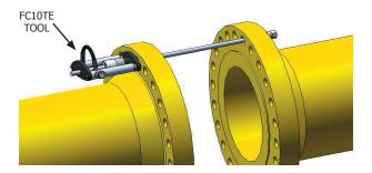
**3.** The ratchet nut is slid over the pull rod and locked into the tool.
