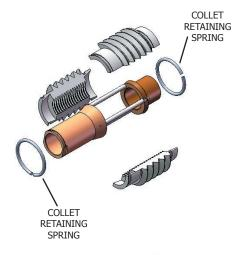
**10.** Clean all components with a rag and WD40 (or similar), removing any visible dirt or grit (paying particular attention to the Collet Segments, Cage and Nut Body).
