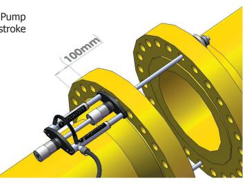
**12.** Release the hydraulic pressure from the system. This will allow the Actuators to retract and the secondary ratchet nut to advance along the pull rod automatically.
