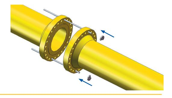
**4.** The Pull Nuts are threaded on to the pull rod.
