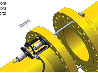
**13.** Once the Actuators have fully retracted close the release valve and continue priming the hand pump untill the actuators have reached full stroke.
