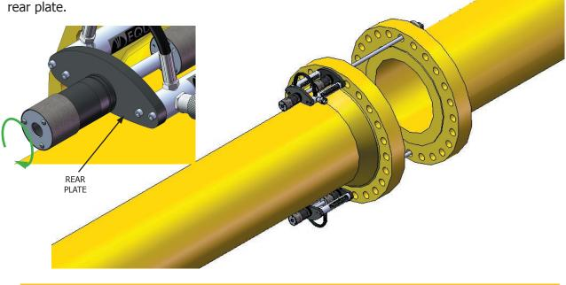
**8.** Check that the release valves on the hand pumps are open by rotating fully anticlockwise and then connect the Pressure gauges to the pump ensuring all the couplers are fully hand tight.
