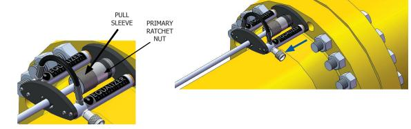
**20.** The Pull Rod complete with pull nut and washer can now be withdrawn from the flange joint.
